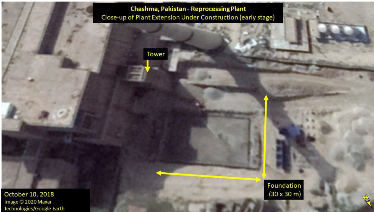
Image. By October 2018, a 30 x 30 m foundation for the extension below ground level is visible in Google Earth imagery.
