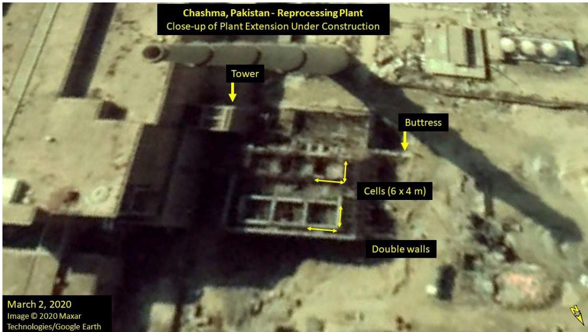
Image. In this March 2020 Google Earth image the layout of one of the upper stories is visible: six cells with double concrete walls, and a hallway.
